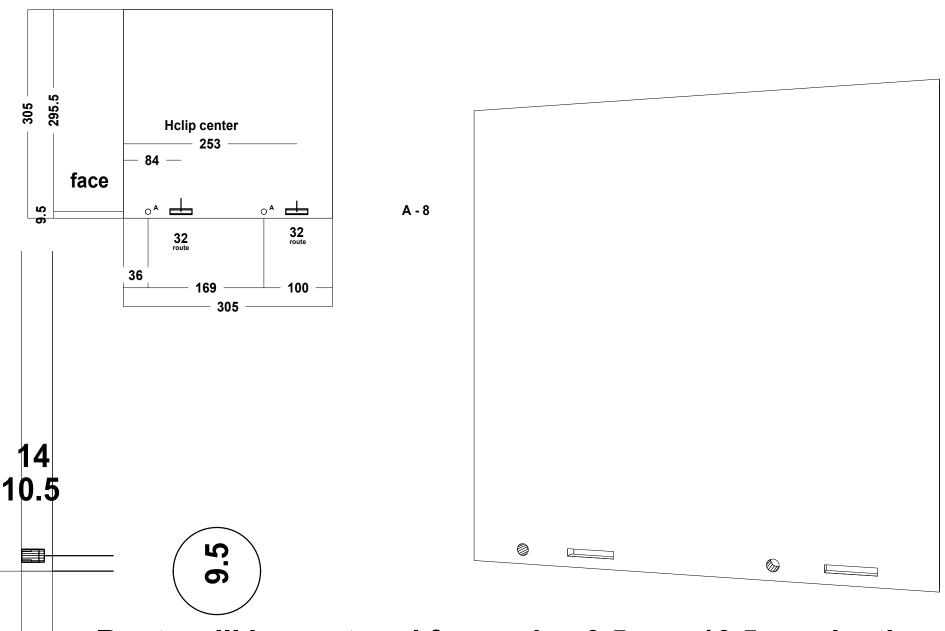
Route will be centered from edge 9.5mm, 10.5mm depth Spring Pin 8mm hole, 14mm depth, also 9.5mm from edge
