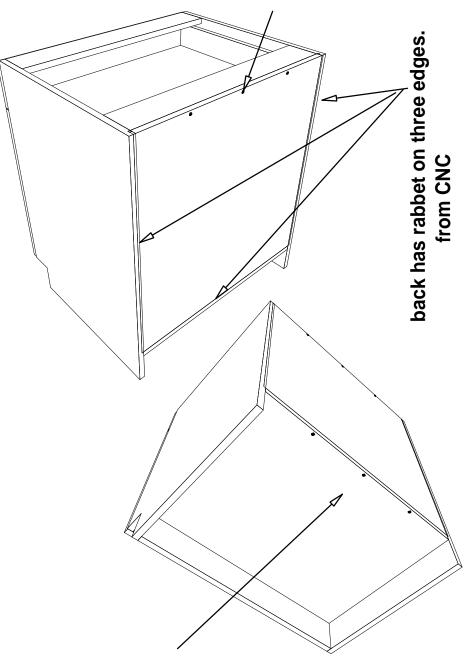
screw deck into bottom edge of 3/4 back.
