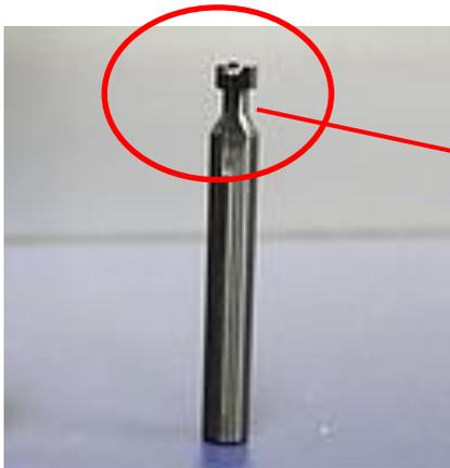
Router bit must be checked every 2,000 cuts
