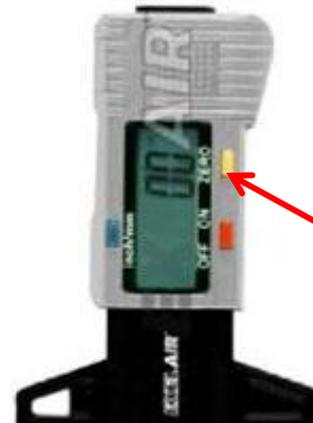
Compress Depth Pin against the panel as shown
